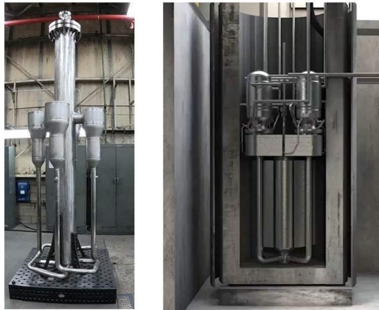
Figure 4.5 MARVEL microreactor. Left: photo of MARVEL; right: illustration of reactor placement in building cavity
